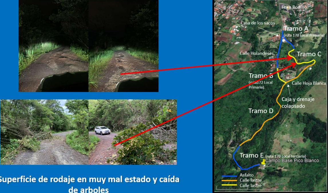
The top-left photograph shows a close-up of a road surface with significant potholes and unevenness. The bottom-left photograph shows a road blocked by a large pile of fallen trees and branches. The map on the right shows five segments: Tramo A (Asfalto), Tramo B (Calle lastre), Tramo C (Calle lastre), Tramo D (Calle lastre), and Tramo E (Calle lastre). A red arrow points from the road damage photos to the corresponding segments on the map.
